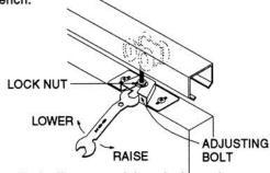
After final adjustment, tighten lock nut down to bracket as shown.
